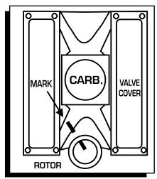
Figure 1 Marking the Rotor Location.
