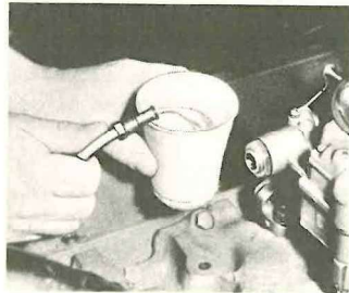
Checking Fuel Flow
